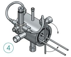
If you need to rotate the spool after it has been inserted, place one rod into the index pin hole and another rod in the slave pilot hole. Use another rod or screw driver to twist the spool into position.
