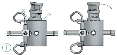
To re-enter a spool for a body that is in the vertical position, lightly lubricate inside of valve near the top. Make sure spool is free of burrs, then rotate the spool so the index pin is in the correct location (see diagrams in catalog). Slot (F) is lined up with discharge port (G) (except in 1300 series). Carefully place edge (A) of the spool into the body then edge (B).
