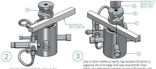
For valves size 12 to 21, place nylon block in spool slot to prevent spool from seriously injuring fingers on edge ICI.
