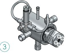
Treating the outside face of the spool like a clock, lightly tap the outer rim (in a precise manner) first at 12 o'clock, then 6 o'clock. If the spool moves slightly at 6 o'clock, then tap again at 12 o'clock, 3 o'clock, or 9 o'clock until the spool moves again. When the spool moves again, remember the last place that was tapped and tap the opposite side of the rim. (If it gets stuck, tap the other end until spool comes out of the body.)
