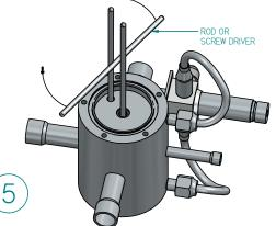
If you need to rotate the spool after it has been inserted, place one rod into the index pin hole and another rod in the slave pilot hole. Use another rod or screw driver to twist the spool into position.
