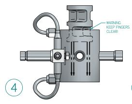
Pull block out of the way. When spool starts to drop, pull hand and fingers clear. Spool will drop suddenly.
